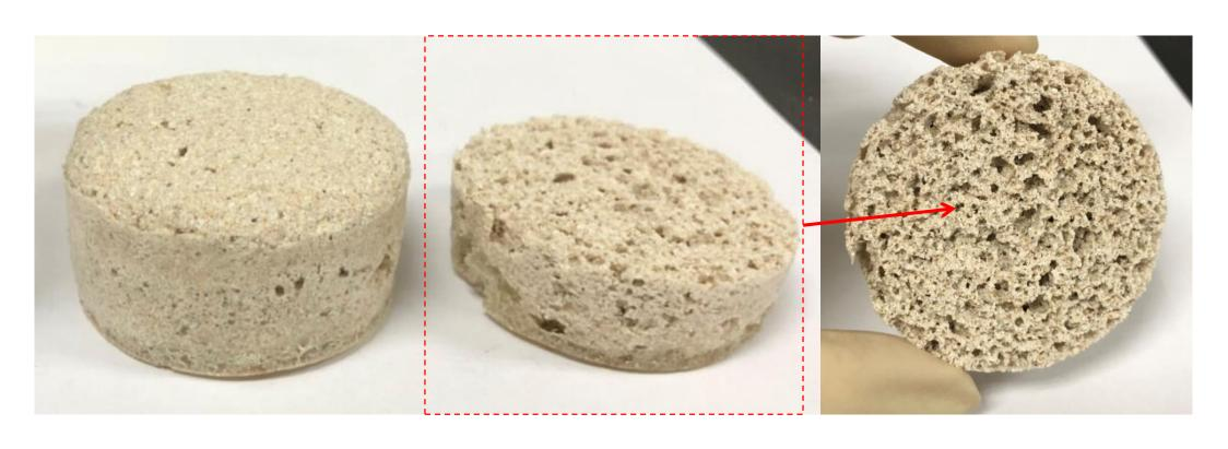
Good thermal stability \( \) fire retardant \( \) low thermal conductivity (k<0.06)
