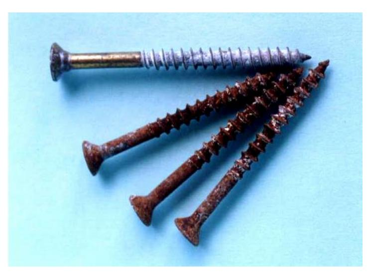
Top 1: Yellow Chromate Znplated steel screw with nano coating showed slight corrosion after 1,000hr. salt spray test.
